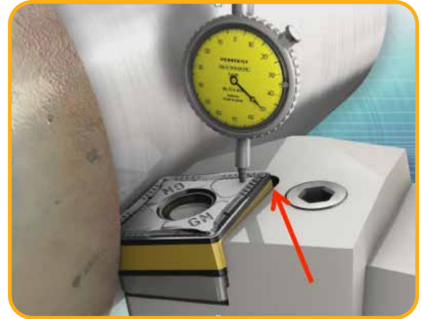
The Cutting Forces Tend to Cause the Standard Insert to Tilt in Standard Lever Clamp Tools
