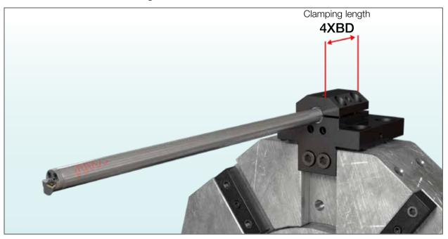
**b** Flat-bed lathe with a tool post provides higher rigidity compared to turret clamping. When using larger diameter bars, the moment exerted on the clamping tool (just by the bars weight) is increased dramatically.
