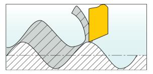
Chatter vibrations are detrimental to the safety and quality of machining operations. They cause a rough surface finish, increase cutting forces, reduce tool and machine life, decrease productivity, and create irritating high noises.
