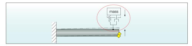
The tuning procedure is performed by experimental modal analysis as shown in the figure below. A modal hammer is used for applying and measuring impact forces and an accelerometer is used for measuring the resulting acceleration. Using these signals, the Frequency Response Function (FRF) which reflects the tool dynamic flexibility is obtained.
