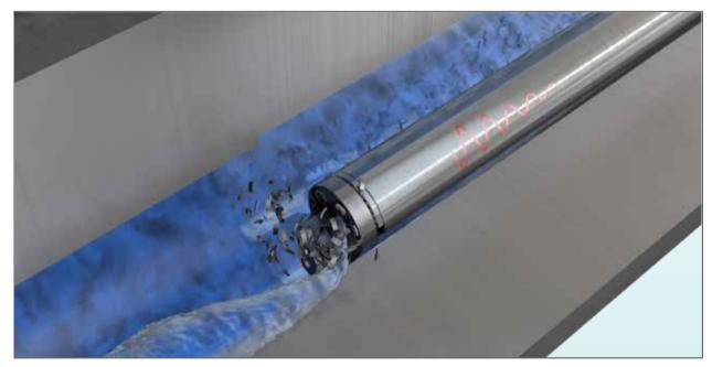
Example: For a bore diameter of 80 mm (3") it is recommended to use a 60 mm (2.5") bar rather than a 80 mm (3") bar. Although the 80 mm bar is stiffer, the lack of space for chip evacuation will decrease the surface finish and can cause breakages.
